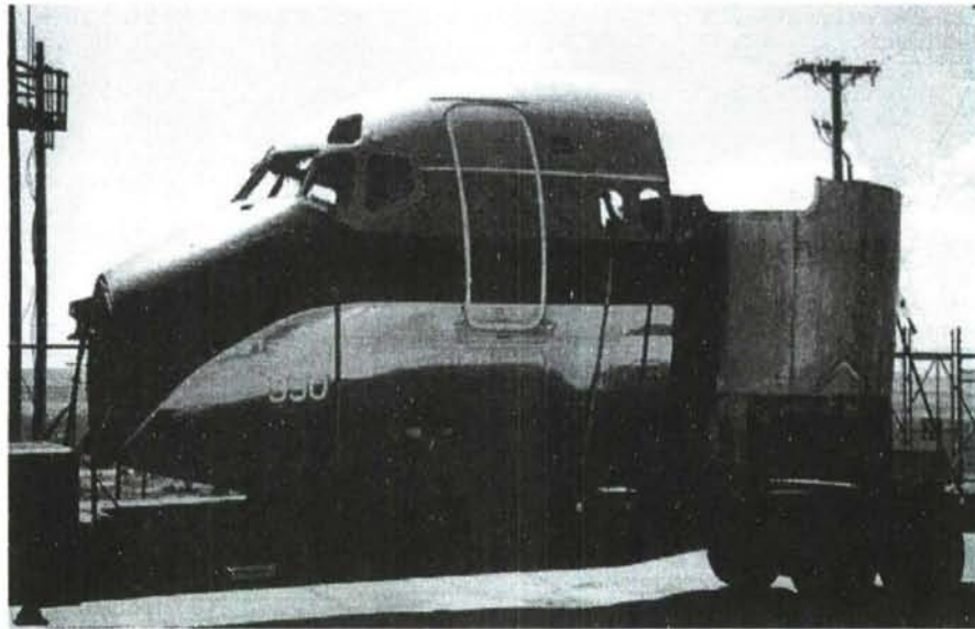
Figure 3. - DC-9 Fuselage Test Specimen (64,360 cycles, 56,520 hours)
