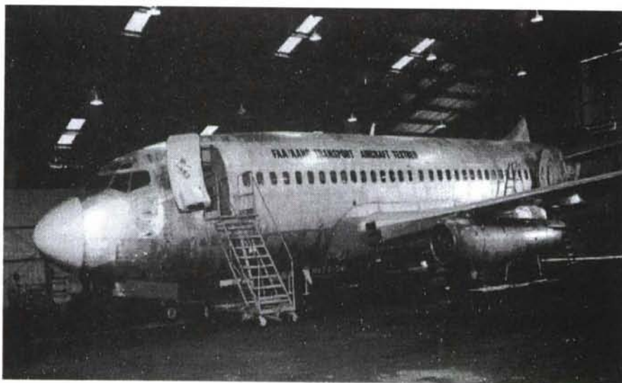
Figure 2. - B-737 Testbed (46,358 cycles, 38,342 hours)
