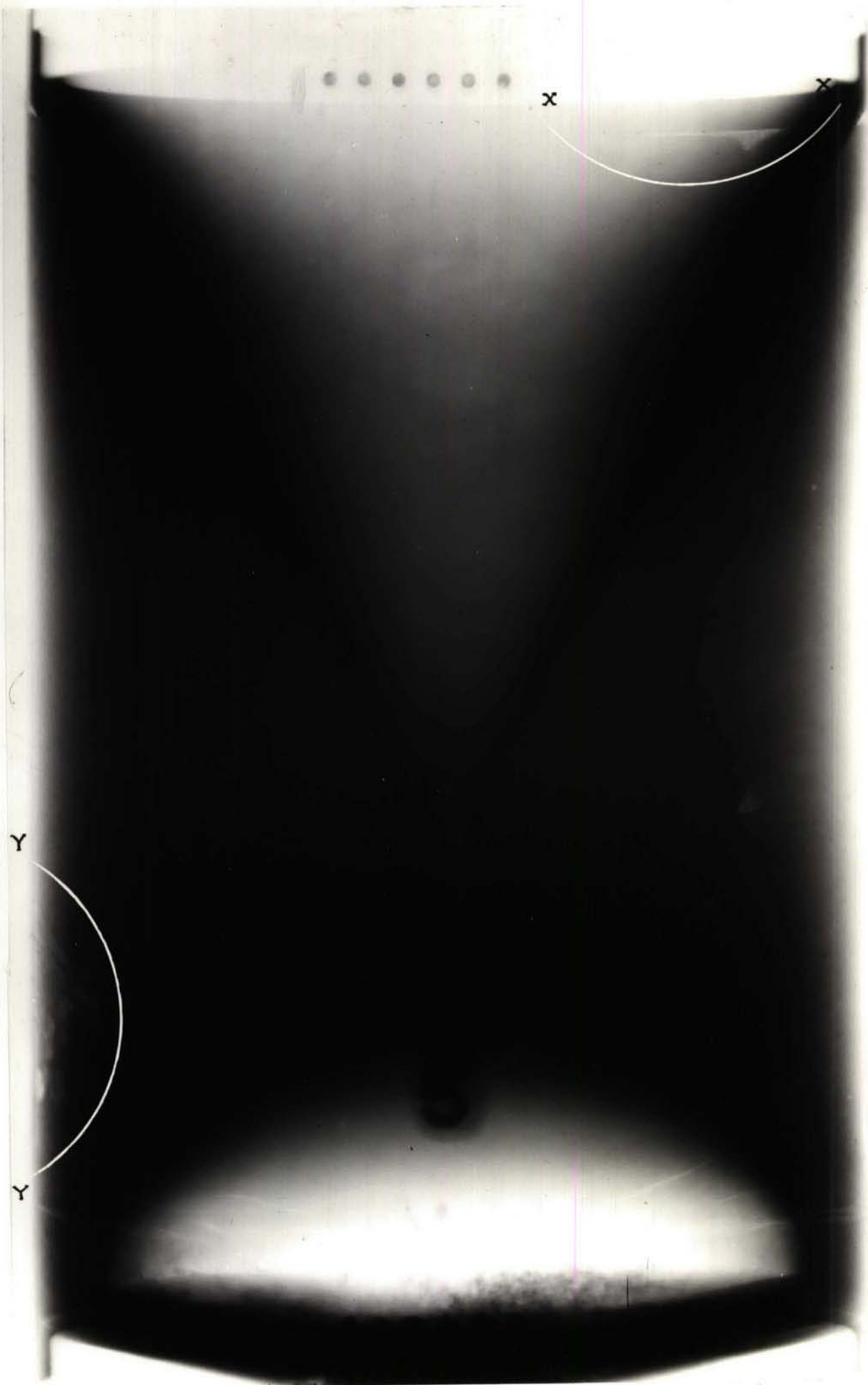
Figure 4 Radiograph of Dart Warhead Area X-X shows discontinuity Area Y-Y shows porosity
