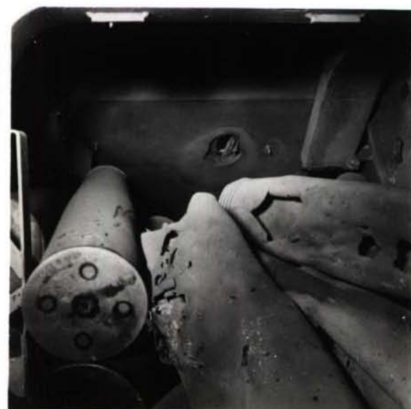
FIGURE 6. TYPICAL JET HOLES AND DAMAGE
