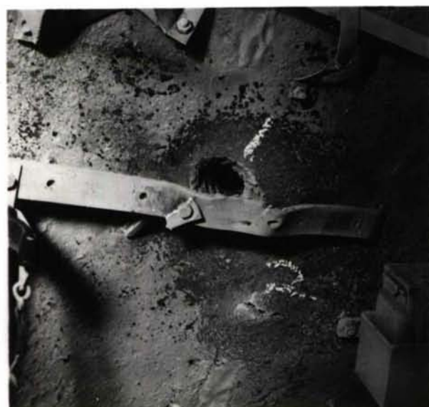
INTERIOR DAMAGE TO ARMOUR BY DART. ROUNDS 1 AND 2
