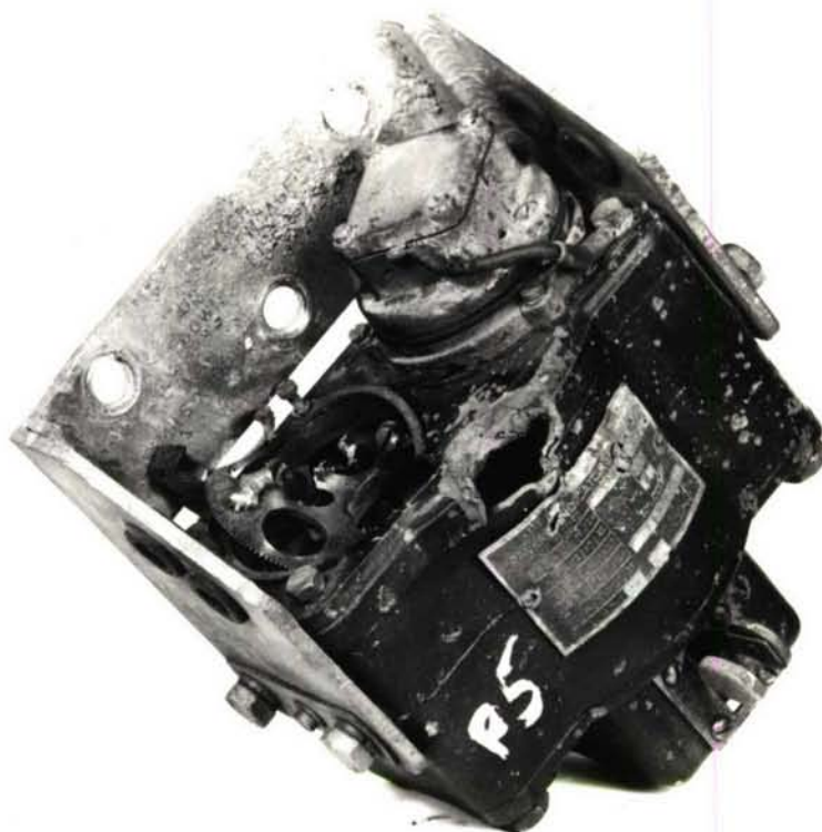
TRAVERSE INDICATOR CONTROL DAMAGED BY ROUND 6
