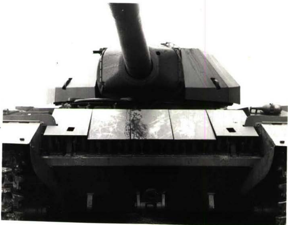
FIGURE 2. CONQUEROR SHOWING SPACED ARMOUR PROTECTION
