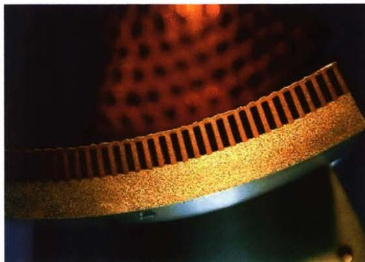
Figure 14: Cut through a combustion chamber wall with CuAgZr liner and galvanic deposited Ni outer shell
