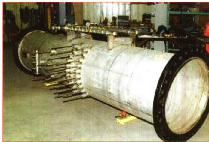
Figure 29. Demonstration MIPCC duct.
