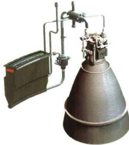
Figure 15. AspiRE cycle based on RL50 engine, Ref.8.
