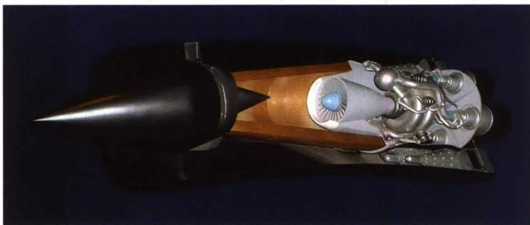
Fig.3. The SABRE engine installed in its nacelle.
