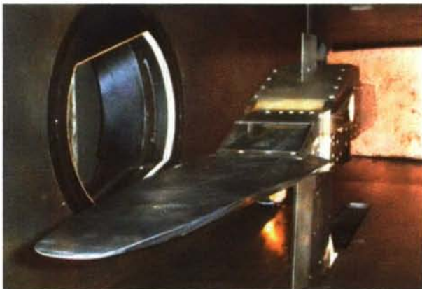
Fig.5 – Mach 2/Mach 8 variable geometry air inlet tested in ITAM wind tunnel
