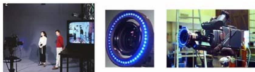
Figure 17: Retroreflective Background and LED-Ringed Camera.
