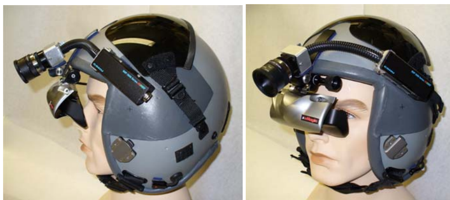
Figure 8: Cohu Camera Mounted on a Gentex Helmet with an NVG Clip.
