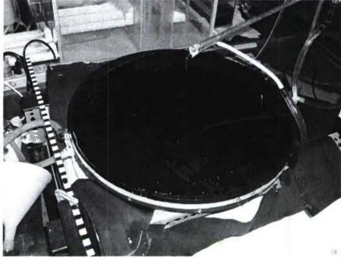
Figure 5: Experimental Setup: A 30 cm diameter plate with a built in manifold is connected to a cooling reservoir and maintained within a degree of freezing. A separate reservoir of fresh water 1^\circ above freezing delivers fresh water at 1^\circ\text{C} to the center.
