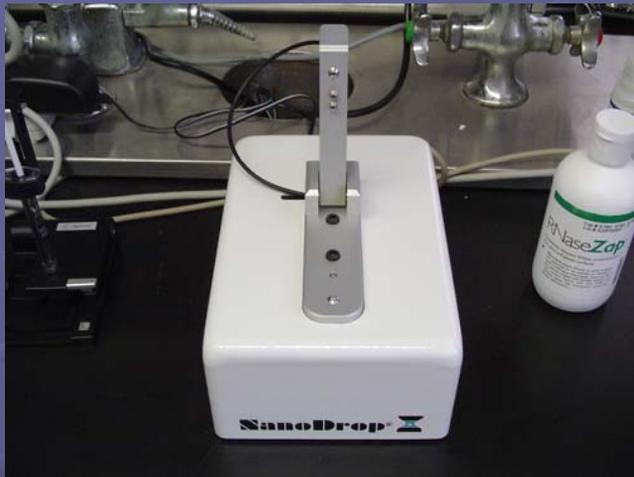
Diode array spectrophotometer
