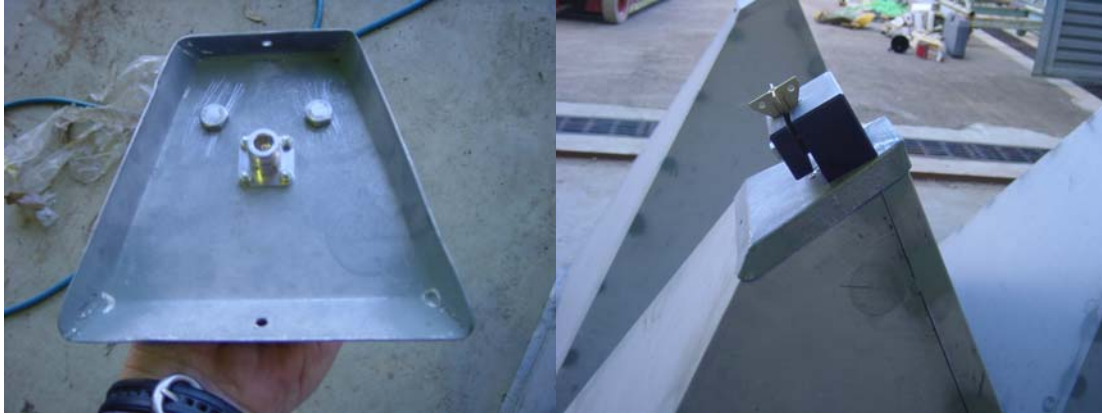
Figure 59 Details of the pyramid apex structure. On the left, the inside of the structure shows the N-connector with earthed outer connected to the sheet metal. On the right, the outside of the structure shows a nylon support block and terminal block connected to N-connector inner conductor.
