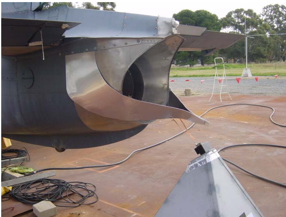
Figure 58 A detail of the sheet aluminium adapter bracket used to electrically connect from the pyramid at the tail to the aircraft jet pipe's existing screws and penetrations.
