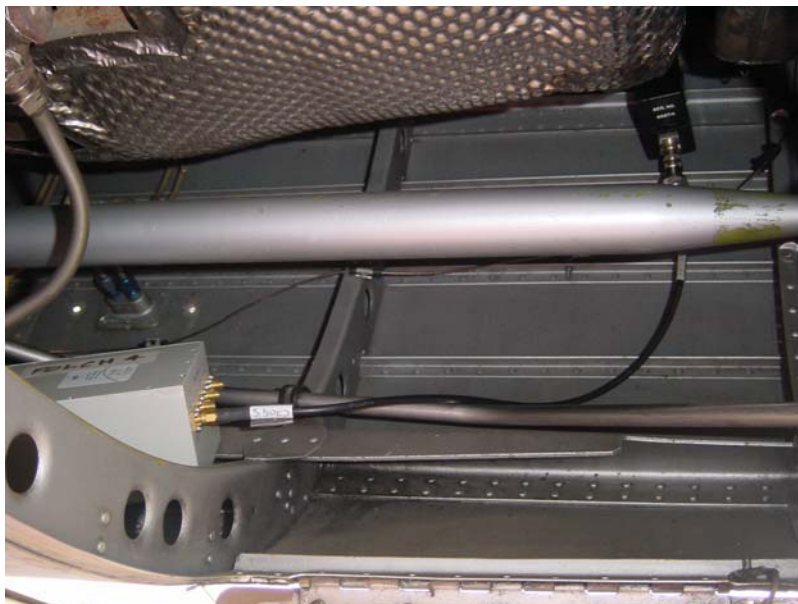
Figure 66 Current clamp location for input 13. It is beneath the jet pipe
