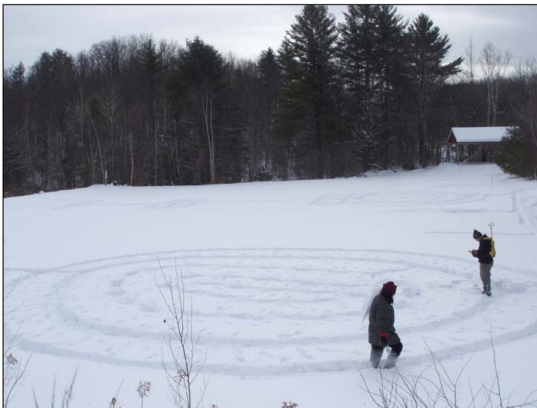
Figure 5. Concentric circle sampling of firing position plume and OTP areas.
