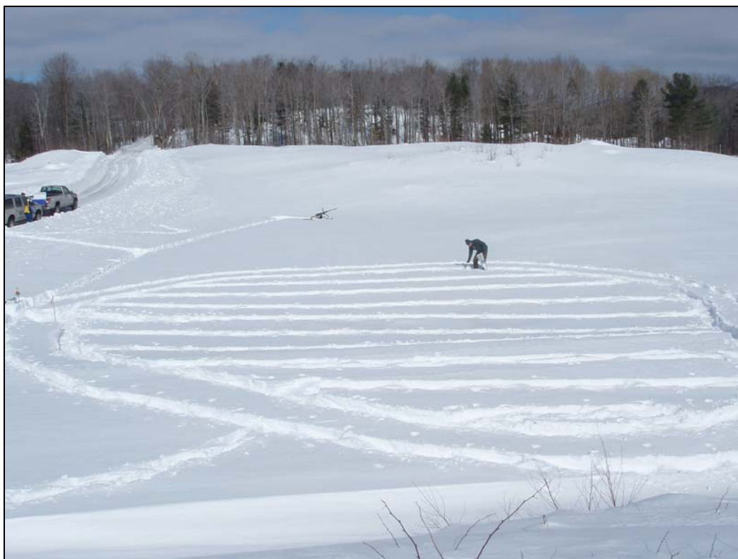
Figure 6. Sampling from fixed lanes in firing position plume area.
