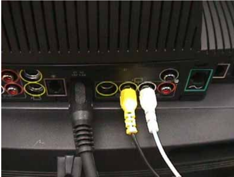
Figure 14. ViewStation power connection
