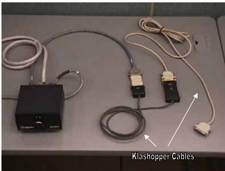
Figure 24. Klashopper cable connection to the switchbox
