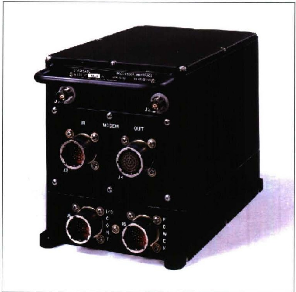
Typical Military EMP Hardened equipment Photo: Ft. Monmouth
