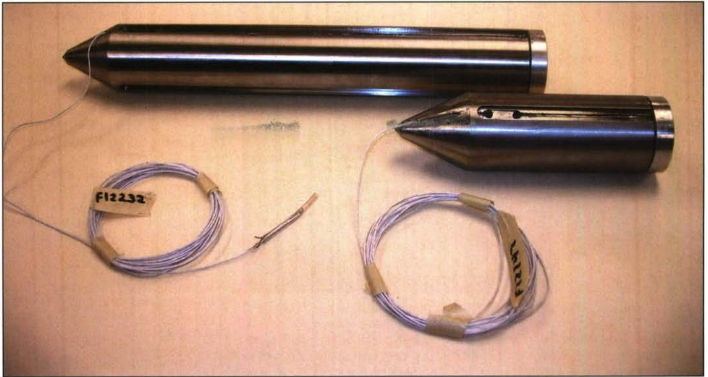
The reaction mass (top) and projectile (bottom) fired from the Davis gun, with accelerometer wires attached to their nose cones. The reaction mass weighed 12.3 lb, and the projectile weighed 3.9 lb. Each had three lengthwise grooves for phenolic resin runners that provided support in the gun barrel and reduced friction. Plastic disks (not shown) at the base ends of the reaction mass and projectile acted as pressure seals.
