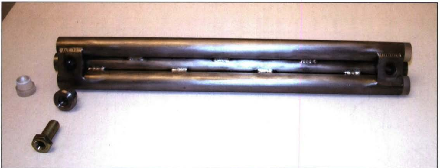
The Davis gun four-tube charge bank assembly. Each tube, loaded with black powder, could be fired independently. The charge bank was 12 in. long and fit inside the 2-in.-i.d. Davis gun.
