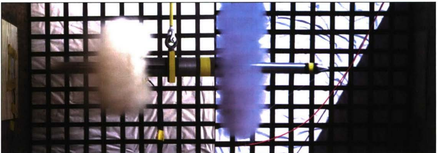
A typical composite high-speed video photograph showing the projectile ( left ) and reaction mass ( right ) just after they exited the Davis gun tube. The black powder gases appear to be of different colors because of differences in the available lighting. The real-time video showed that the Davis gun exhibited little to no pendulum motion during the five test shots, indicating that the momentums of the projectile and reaction mass were balanced.
