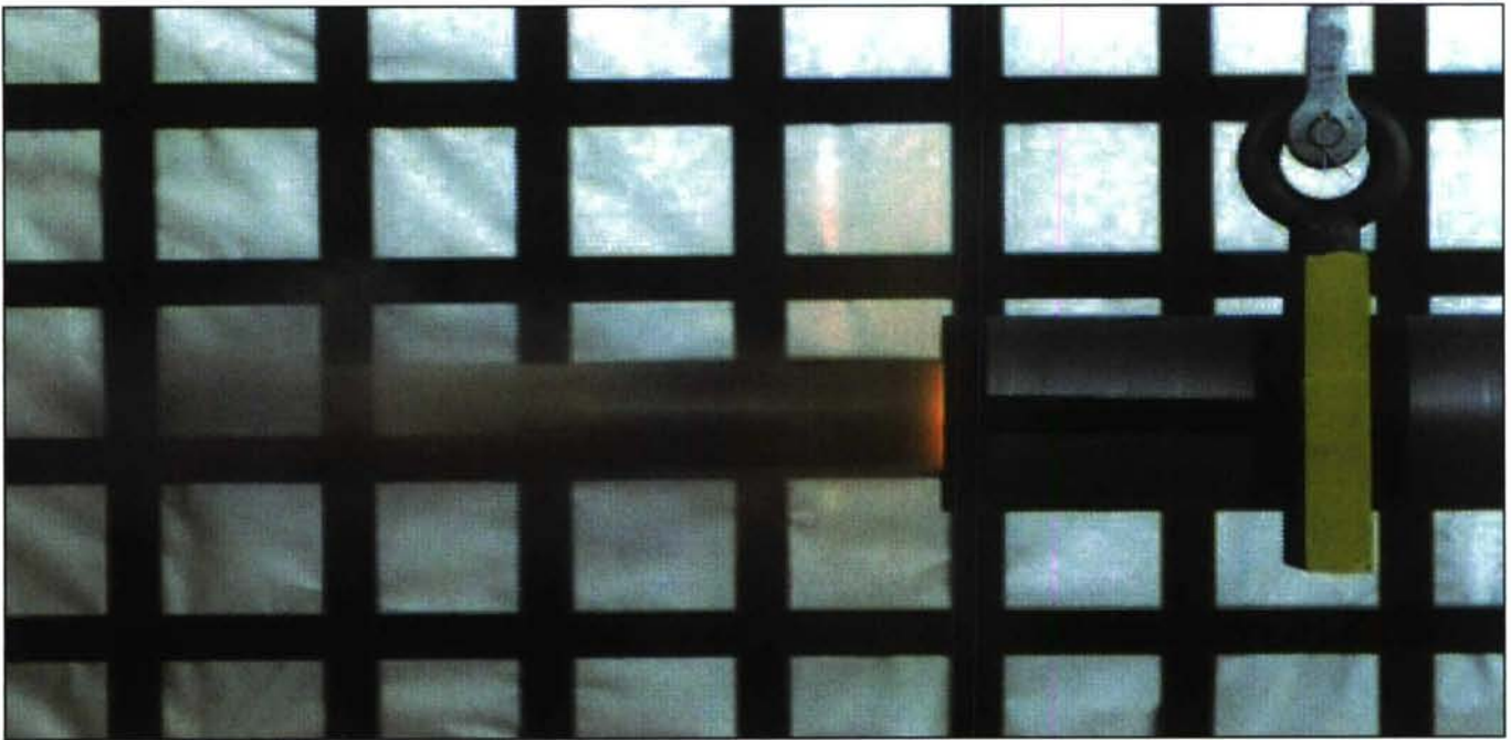
Video photograph showing the projectile as it exited the Davis gun tube. The shroud of hot propellant gases enveloping the projectile made video measurements difficult: in fact, the reaction mass provided better measurements because its nose cone already protruded from the gun barrel before firing and so traversed clear air ahead of propellant gases.
