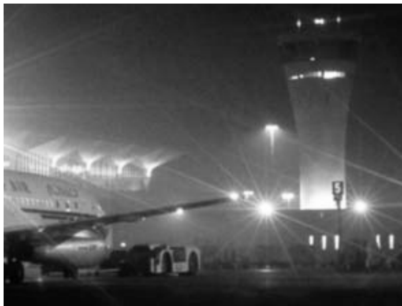
Figure 9: Glare from airport ramp lighting.
