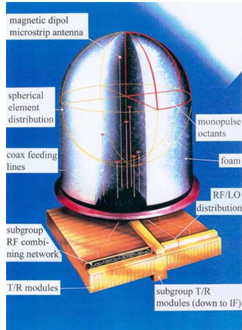
(b) Concept of radar with Crow's Nest antenna
