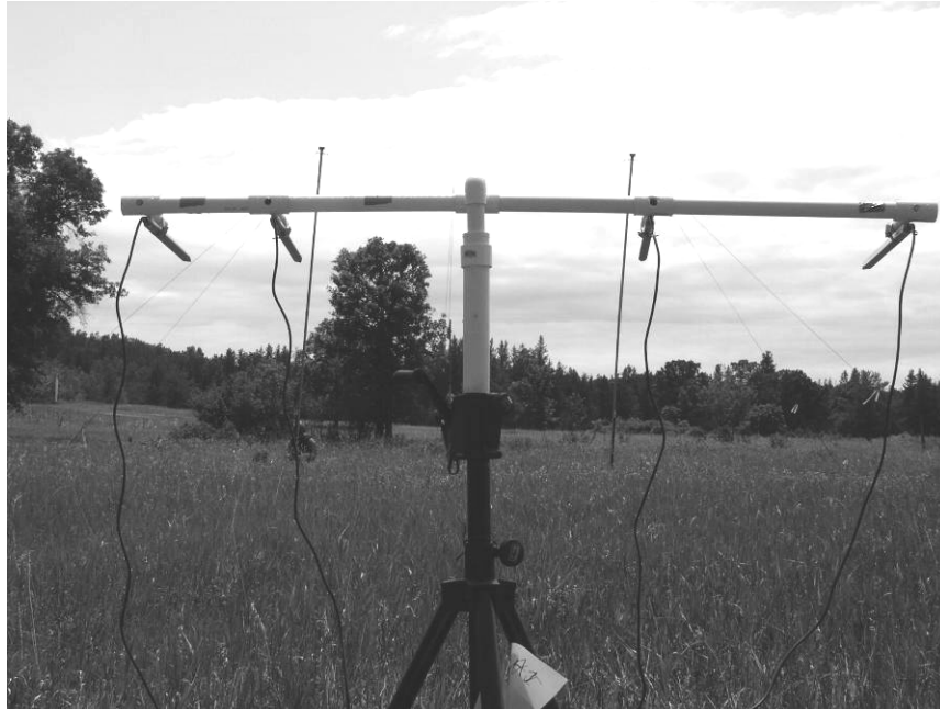
Figure 4. A microphone array is shown in the parallel configuration.
