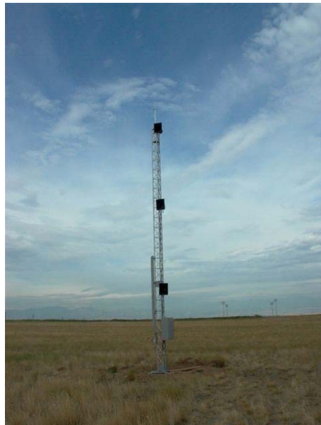
Figure 2: A source tower of the acoustic tomography array.
