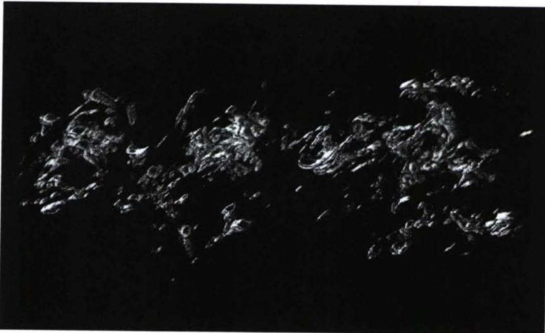
Fig. 22 Reconstructed and shaded 3-D image for Run 003.  $U = 5.22$  cm/s. The center of the field of view is located 65.3 cm downstream of the turbulence-generating grid where the dye filament is released.
