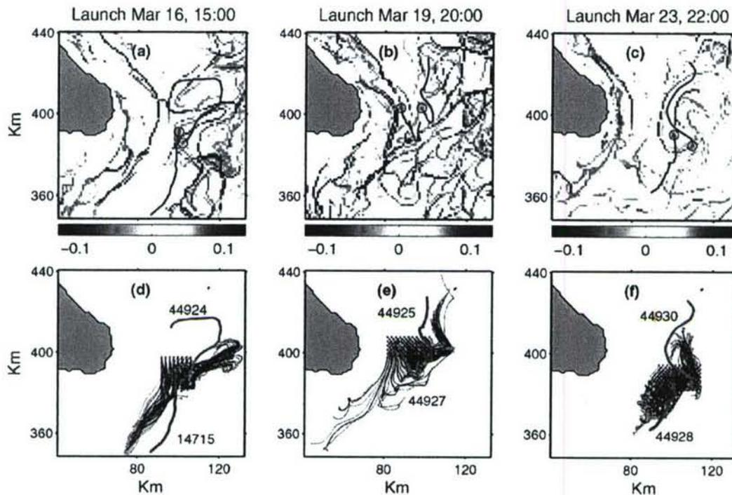
**Figure 3.** The initial 2-day trajectories for real (gray in top panels, green and purple in bottom panels) drifters launched on March 16, March 19, and March 23 (launch position indicated by circles). Superimposed are (a, b, c) the FSLE ( $\delta_i = 0.45$  km and  $r = 40$ ) computed at launch time, and (d, e, f) synthetic drifters released in regular arrays. Red (blue) dots indicate initial (final) positions of the synthetic drifters.
