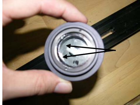
Figure 20. Sample 19 did not fill the sample holder window and was rejected.
