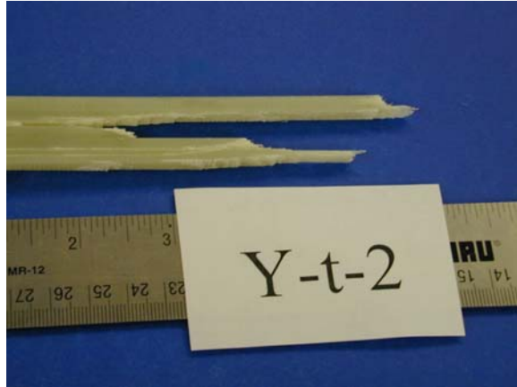
Figure 10. Photograph showing failure mode; Specimen Y-t-2.
