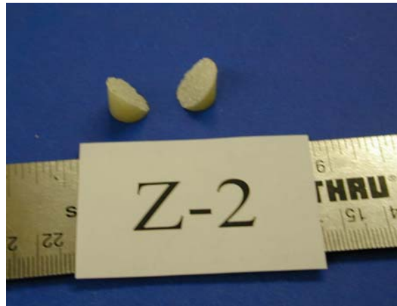
Figure 7. Photograph showing failure mode; Specimen Z-2.
