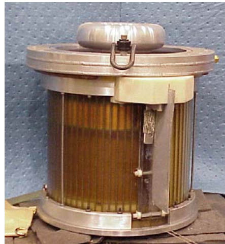
Figure 8. Line schematic and a photograph of the pulse transformer to step up the voltage from 50 kV to over 1 MV
