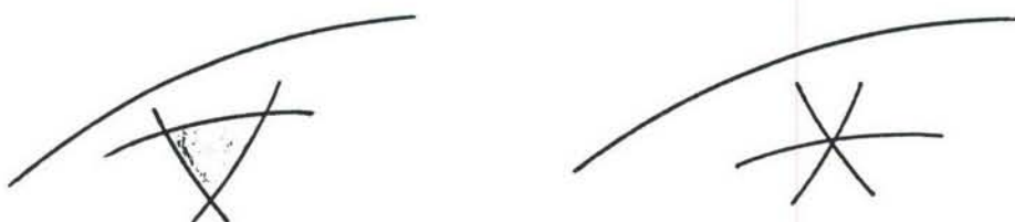
Figure 4. Intersections of three position lines before and after clock corrections. See descriptions of Omega and Global Positioning System.
