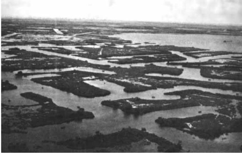
Figure 54 Canals dug in Louisiana's coastal marshes for oil and gas drilling and production operations.
