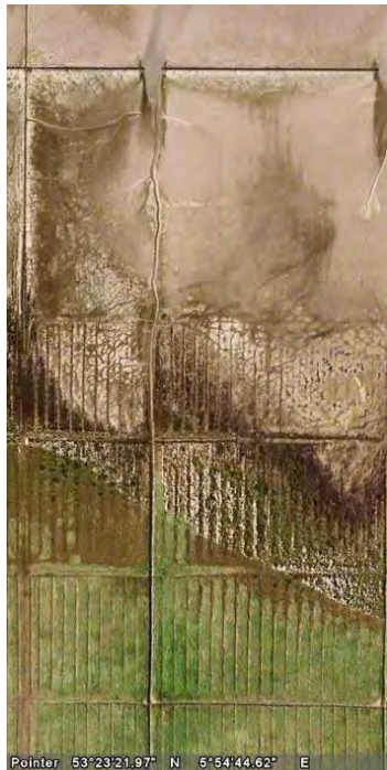
Figure 28 Aerial picture showing large-scale marshland (" kwelder ") creation and stabilization works using low tech measures. The muddy area and marsh vegetation are flooded each tidal cycle (Dutch Wadden Sea, source: Google).
