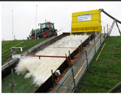
Figure 27 Recent field test in the Netherlands on the impact of overtopping waves on an existing levee.
