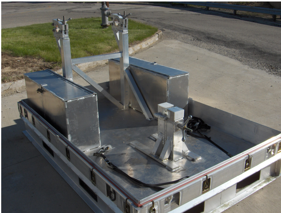
Figure 2. Two aft clamps and one forward clamp hold the gear in place. Nylon straps prevent the tires from rotating.
