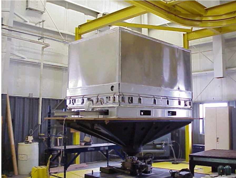
Figure 13. Vibration Testing Set-up (difference between Resonance Dwell and Repetitive Shock tests indistinguishable by photograph). .
