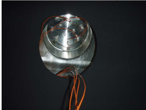
Figure 25: Connection of 2 nd Set of Thermocouple Wires to Right Wiring Interface Inside Chamber
