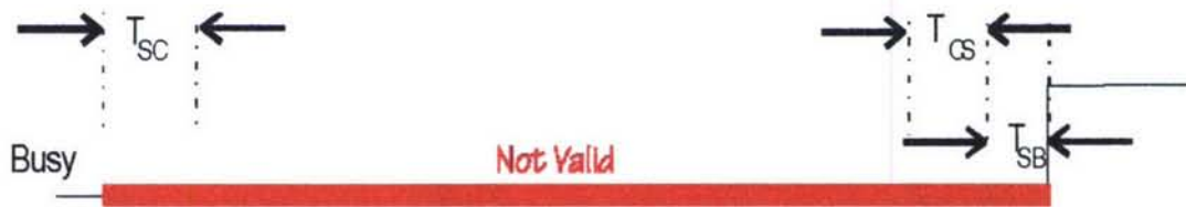
Figure 3: Micro Lambda's timing illustration. T_{sc} > 2 \text{ usec} select low before first clock, T_{cs} > 2 \text{ usec} clock low before chip select high, T_{su} > 2 \text{ usec} data stable before rising edge of clock, T_{ch} > 2 \text{ usec} minimum clock high time, T_{cl} > 2 \text{ usec} minimum clock low time, T_{sb} > 10 \text{ usec} (time to wait before sampling 'BUSY' Data and Clock setup / hold time = 10 usec. {hold time is determined from T_{ch} })
