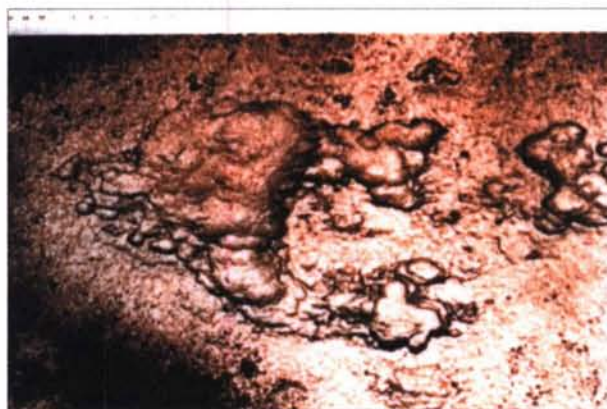
FIGURE 7. Close-up of sand-blasted surface showing MIC pattern. 52 Reproduced with permission from The Gas Technology Institute.
