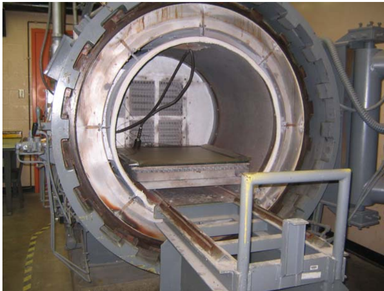
Figure 11. Autoclave setup which was used to fabricate the laminates (at AFRL facility)
