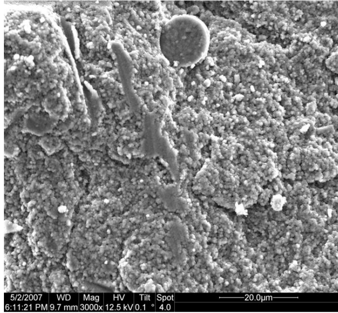
Figure 168: Side of the fracture surface of the N720/A specimen tested in -6.5 MPa creep in steam at 1200^{\circ}\text{C} .
