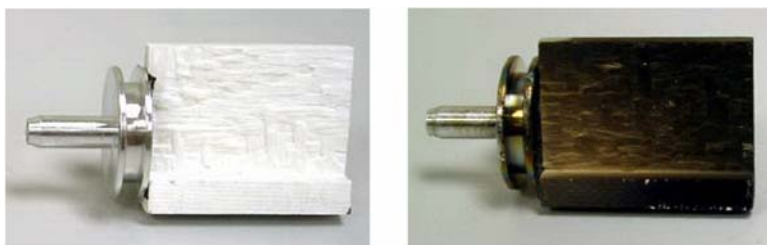
Figure 26: A specimen fracture surface before and after carbon coating.
