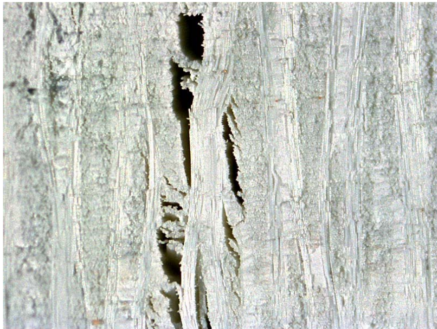
Figure 104: Close-up of the midplane of the N720/A specimen tested in creep at -5.0 MPa at 1200 °C in steam for 100 h.
