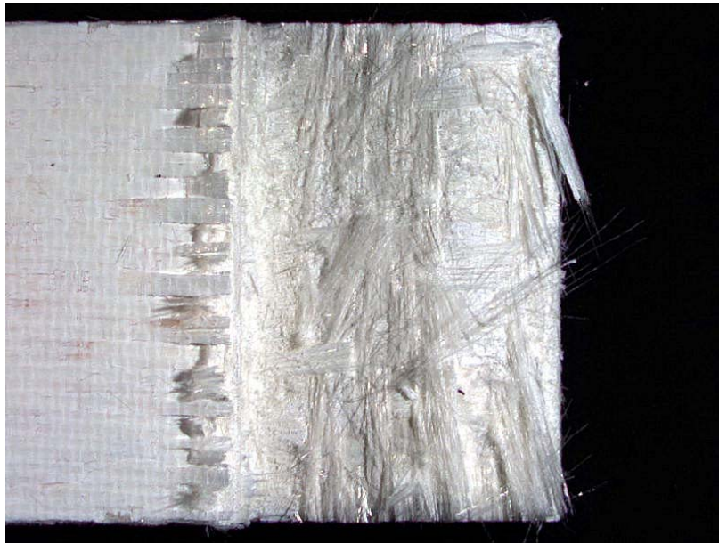
Figure 75: Side views of fracture surfaces of N720/A specimen tested in tension to failure at 1200 °C in air. (a) is of Piece A. (b) is of Piece B.
