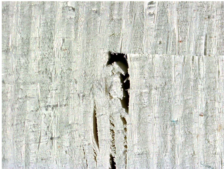
Figure 48: A close-up view of the closed notch of the N720/A specimen tested in creep at -5.0 MPa for 100 h at 1200°C.
