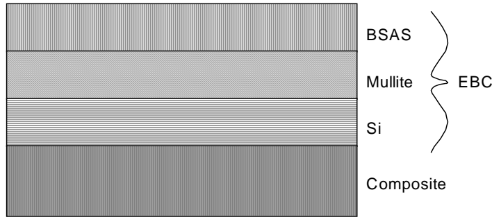
Figure 1: Typical three layer EBC used in combustor liners.
