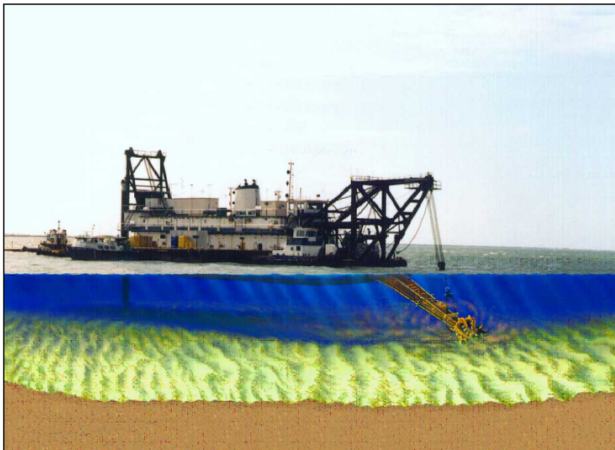
Figure 11. Hydraulic cutterhead pipeline dredge.
