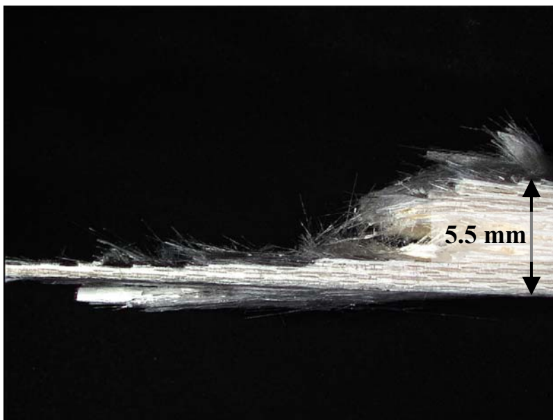
Figure 225. Fracture surface of N720/A specimen tested in compression to failure in steam at 1200°C in displacement control at -0.05 mm/s.
