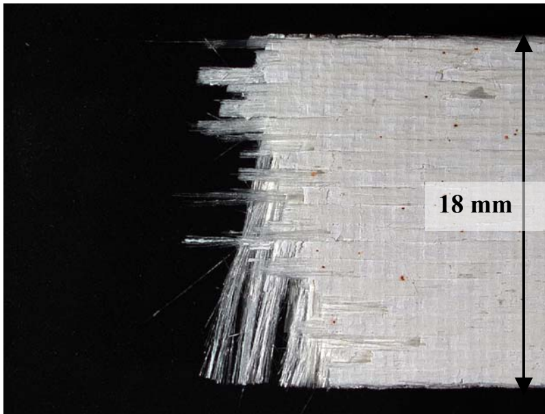
Figure 188. Fracture surface of N720/A specimen tested in compressive creep at -60 MPa for 100 h at 1200°C in air.
