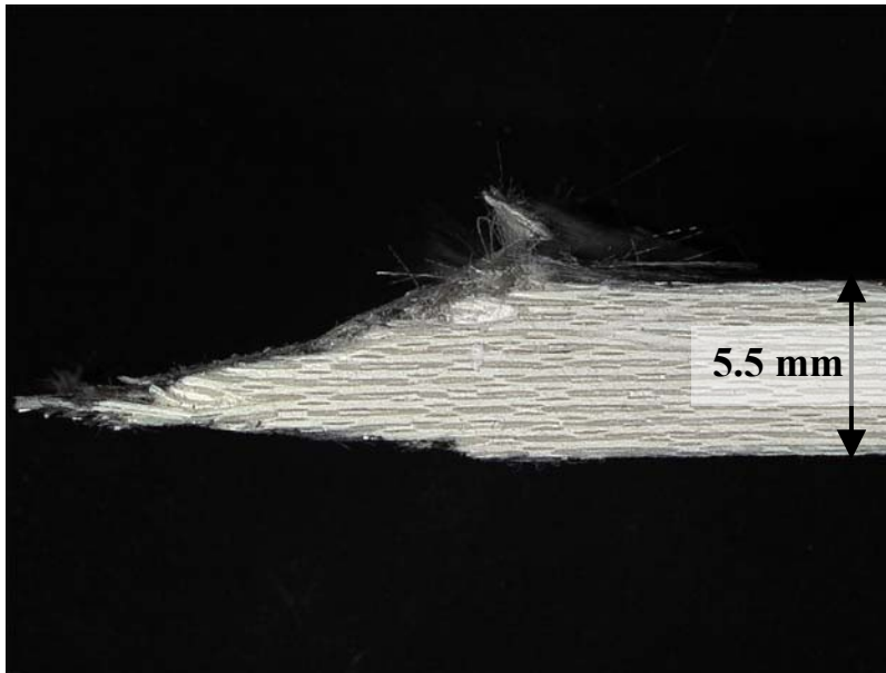
Figure 193. Fracture surface of N720/A specimen tested in compressive creep at -100 MPa for 100 h at 1200°C in steam.
