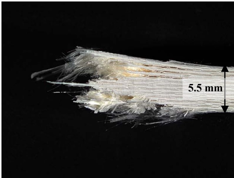
Figure 218. Fracture surface of N720/A specimen subjected to aging in steam at 1200°C for 25 h then failed in compression.
