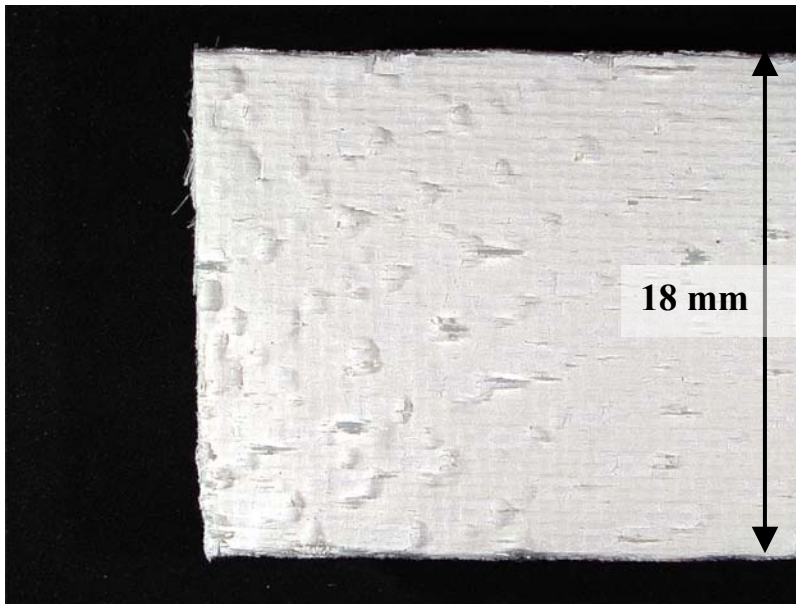
Figure 238. Fracture surface of N720/A specimen tested in compression to failure in steam at 1200°C in stress control at -0.0025 MPa/s.
