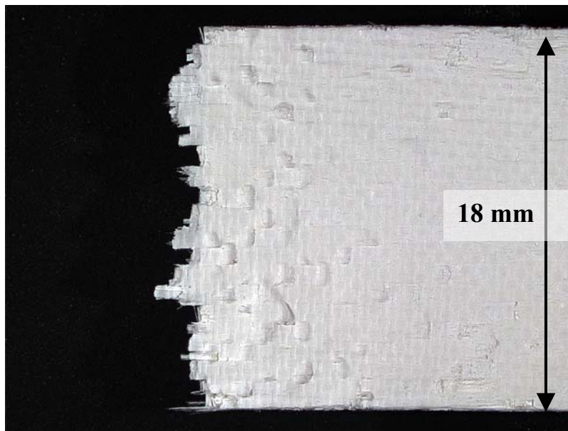
Figure 242. Fracture surface of N720/A specimen tested in compression to failure in steam at 1200°C in stress control at -0.0025 MPa/s.
