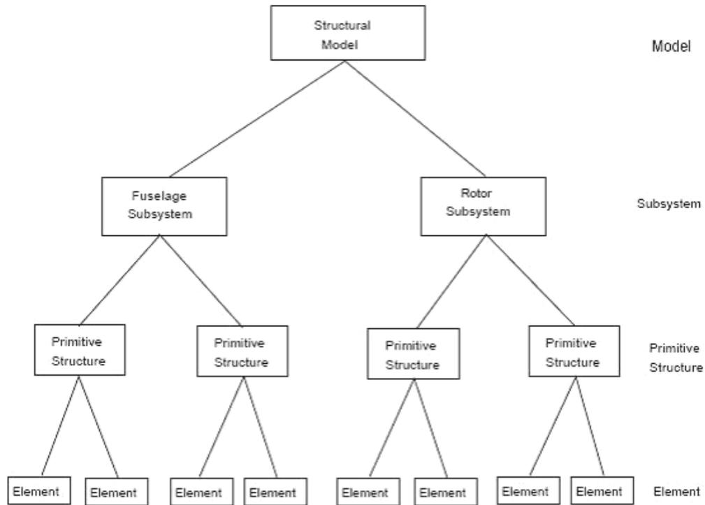
**Figure 8. Block Diagram of the Structural Model (6)**
