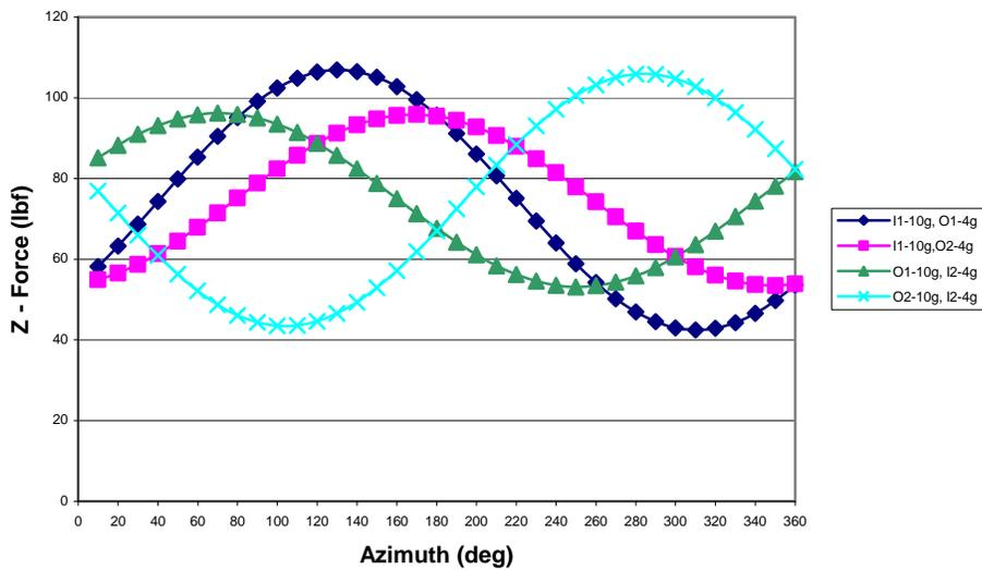
**Figure 29. Apache Rotor System 10g-4g Adjacent Blades**
