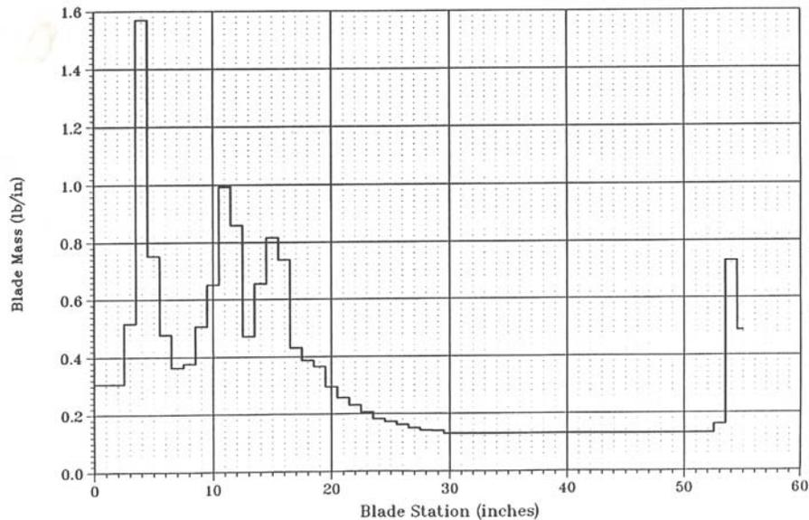
**Figure 12. Apache Tail Rotor Blade Mass Distribution (8)**
