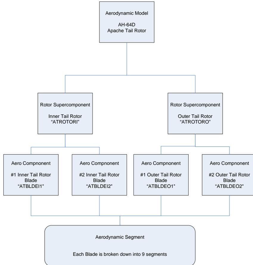
**Figure 18. AH-64 Apache Tail Rotor Aerodynamic Model**
