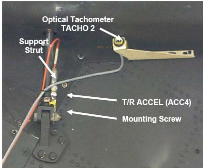
**Figure 5. Accelerometer and Tachometer Installation locations. (17)**
