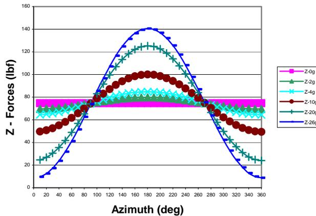
**Figure 20. Traditional – Multiple Weights, Single Blade – Z forces**
