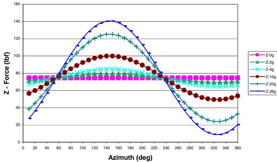
**Figure 21. Apache – Multiple Weights, Single Blade**
