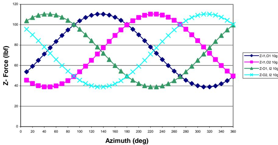
**Figure 26. Traditional Equal wt (10g) to Adjacent Blades**
