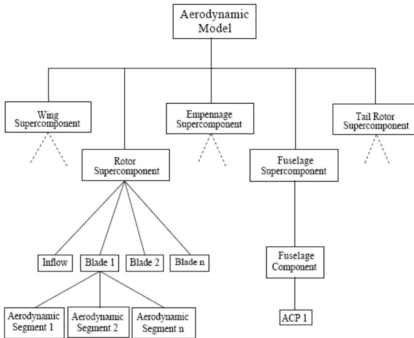
**Figure 9. Aerodynamic Model Hierarchy (6)**
