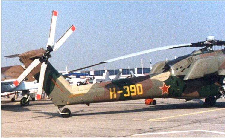
**Figure 3. MIL MI-28 Scissor Tail Rotor Variant**
