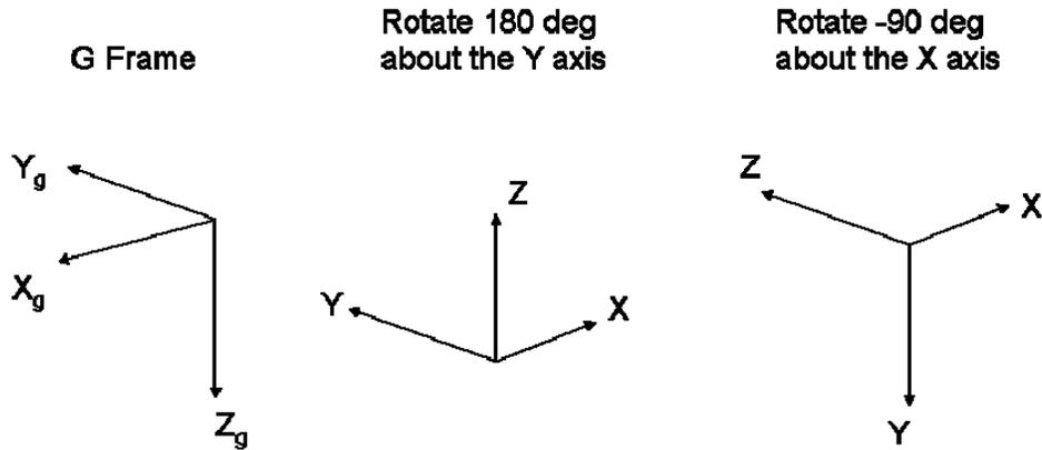
**Figure 11. Rotational Sequence of the Tail Rotor Subsystem**
