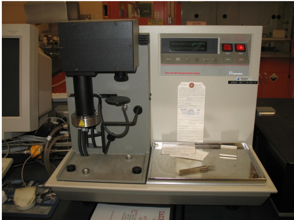
Figure 3: TA Instruments Hi-Resolution TGA-2950 Thermo-Gravimetric Analyzer
