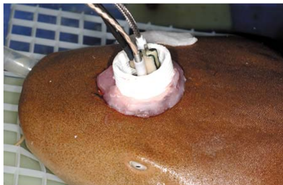
Figure 21: Two sixteen-channel x1 headstages (Tucker-Davis Technologies) allow semi-chronic access to the electrode arrays through a waterproof housing (partially shown).
