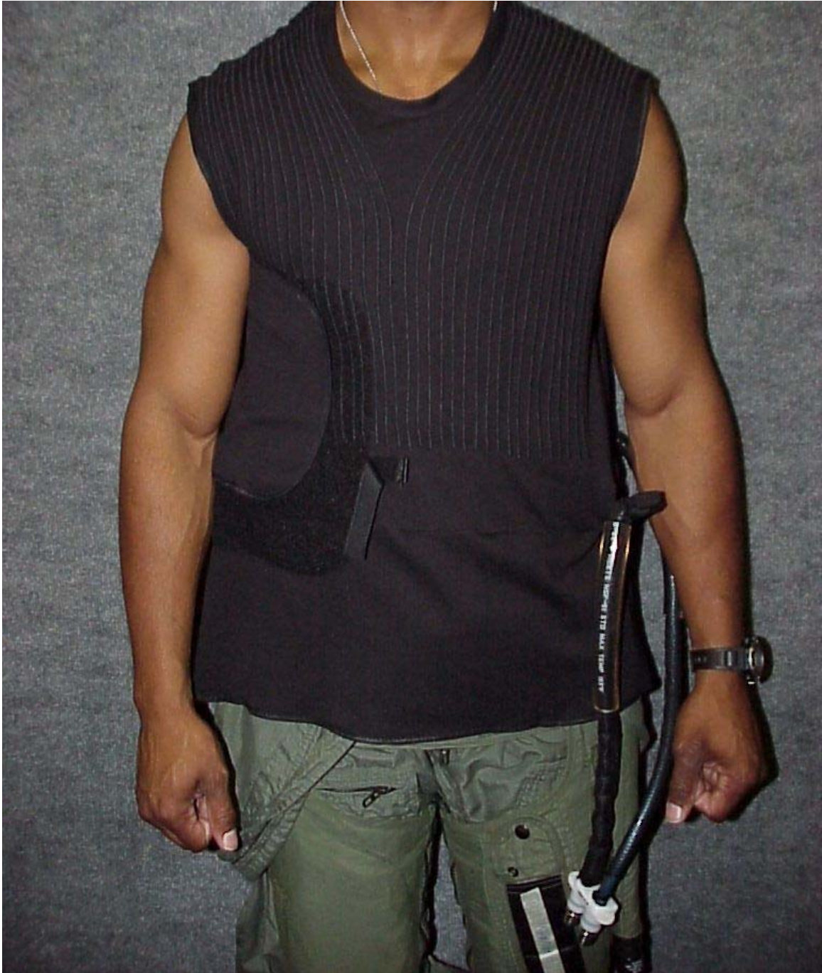
Figure 2. The Liquid Cooling Vest with connecting liquid hoses on the subject's left side.
