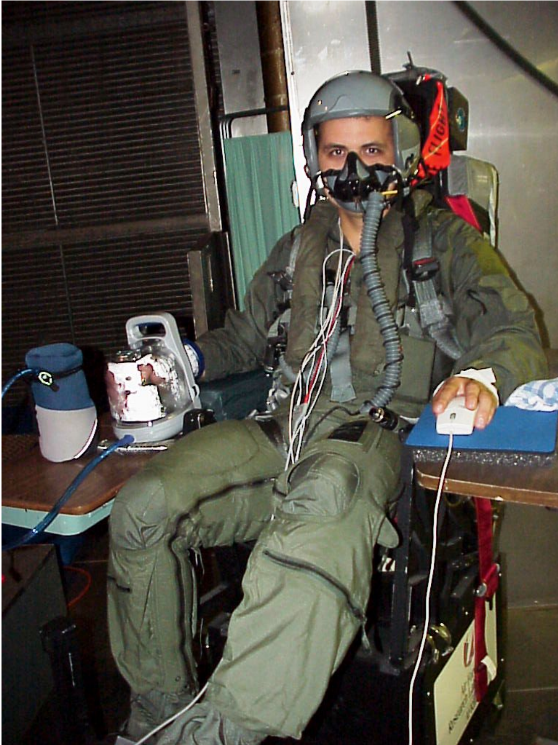
Figure 3. Subject with his right hand in the Rapid Rapid Thermal Exchange (RTX®) hand cooling device in the thermal chamber. The left hand is moving the mouse for the responses in the computer operated cognitive performance tests.
