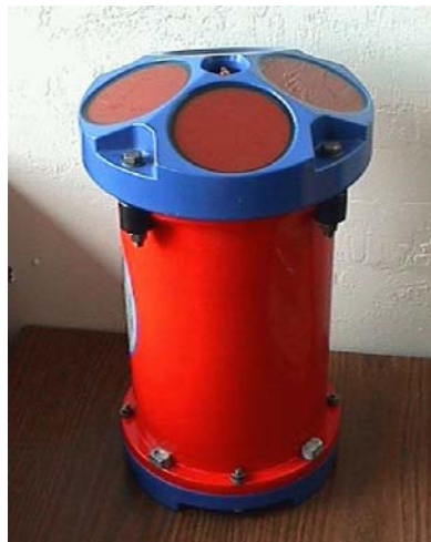
Figure 15. Workhorse Monitor Acoustic Doppler Current Profiler (ADCP) mounted on the MISO instrument frame. Manufactured by RD Instruments. (From Stanton 1998)
