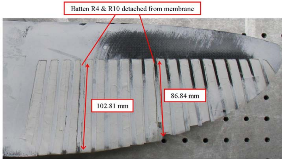
Figure 15: Test 1, Right Span Wing Damage
