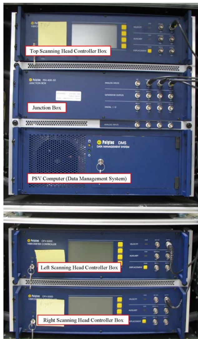
Figure 6: PSV Controllers, Junction Box, and Data Management System
