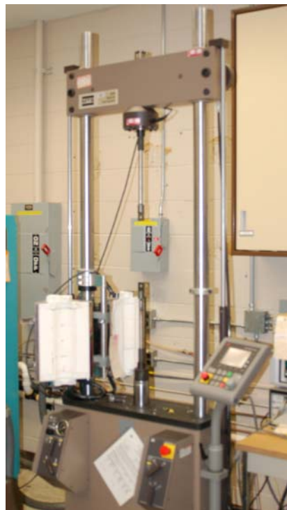
Figure 3.16: MTS 810 Material Test System used to obtain tensile property data.
