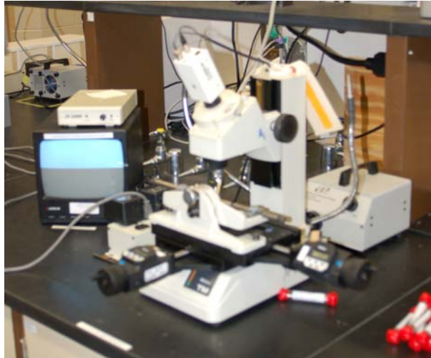
Figure 3.15: Mitutoyo machinist microscope used to make fatigue and CT specimen measurements.
