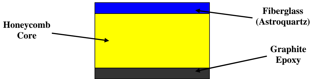
Figure 5: Conformal Load-Bearing Antenna Structure Cross-Section
