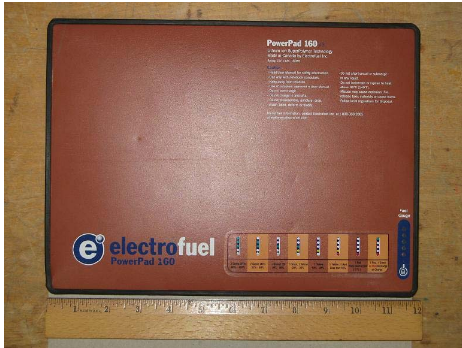
Figure 18. 15VDC, 11000mAh, rechargeable Lithium Ion battery.
