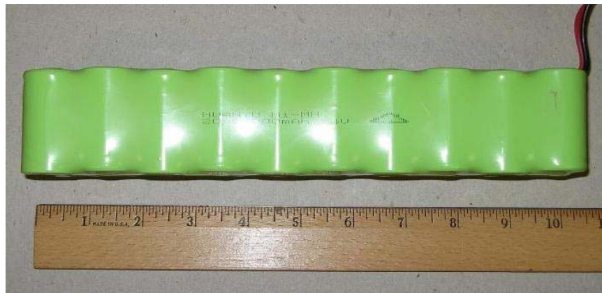
Figure 17. 20 cell, 24VDC, 4000 mAh, rechargeable NiMH battery pack.
