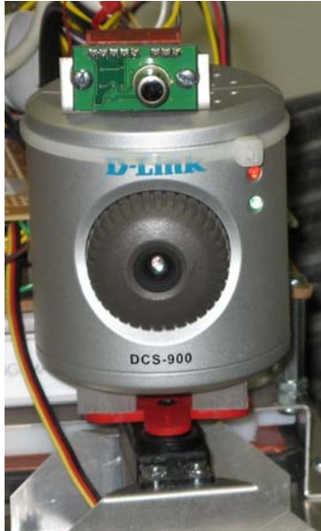
Figure 34. Thermal Sensor Mounted on Camera.
