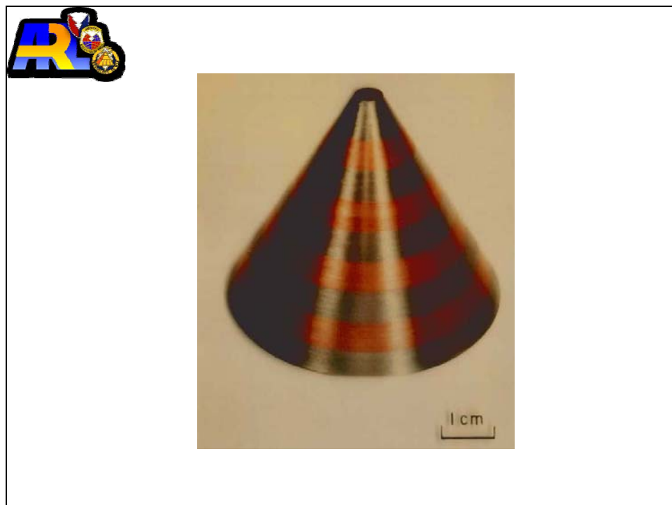
Figure 103. Finish-machined alternately layered copper-nickel cone.
