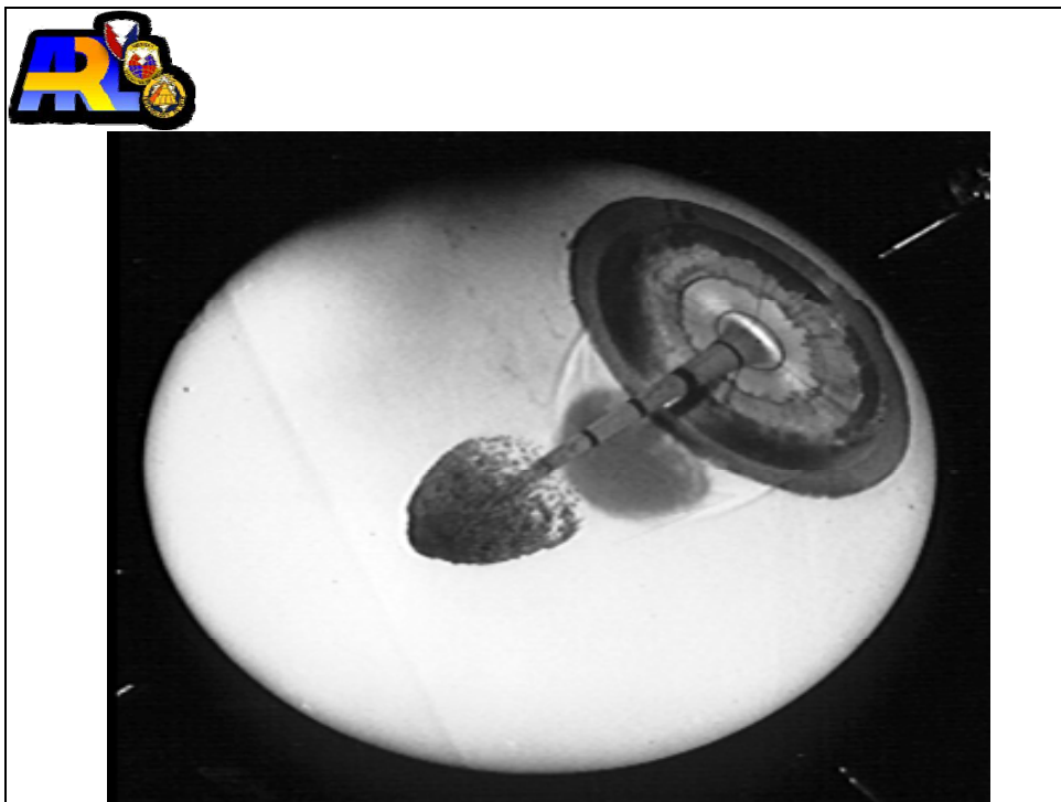
Figure 19. High-speed camera viewing the collapse of a shaped charge with a conical liner (continued).
