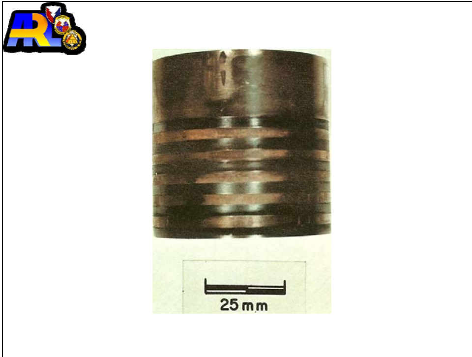
Figure 92. Diffusion-bonded alternately layered copper-nickel cylinder.
