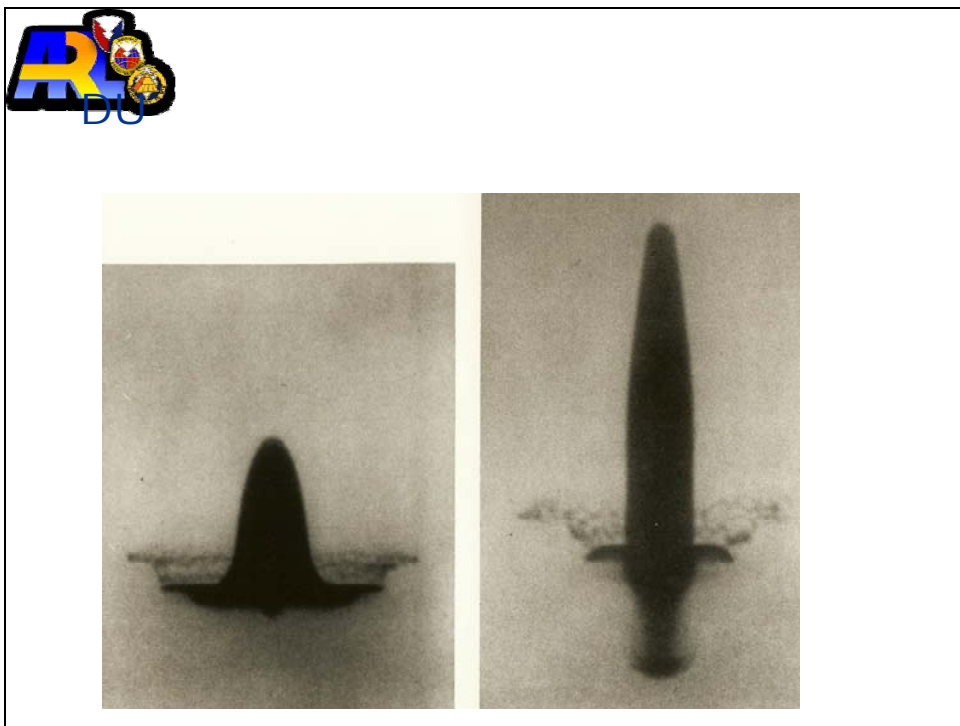
Figure 143. Early time collapse of a hemispherical depleted uranium liner.
