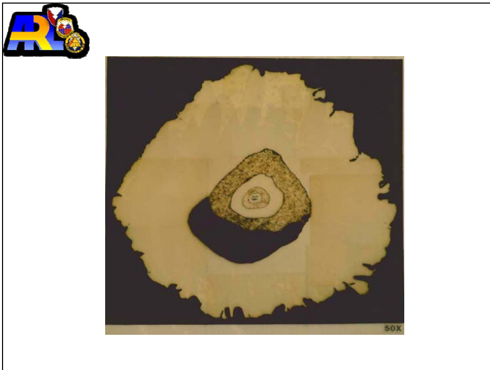
Figure 97. Cross section of jet particle from alternately layered copper-nickel hemispherical liner.
