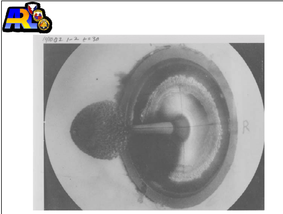
Figure 18. High-speed camera viewing the collapse of a shaped charge with a conical liner (continued).
