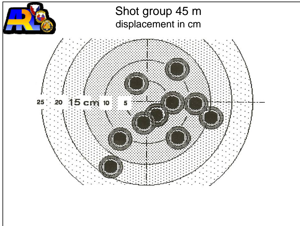
Figure 128. Hit precision of EFP with star-shaped tail at 45 m. The displacement was less than 20 cm.
