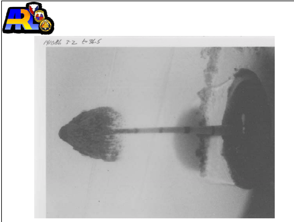
Figure 20. High-speed camera viewing the collapse of a shaped charge with a conical liner (continued).
