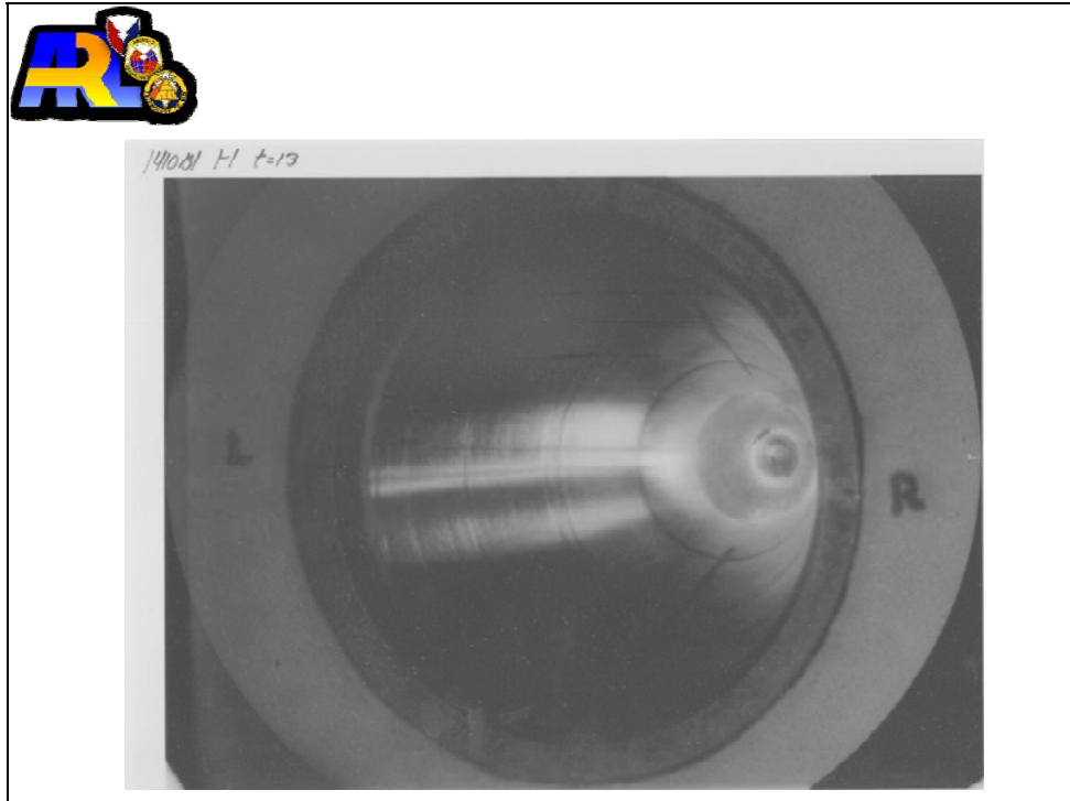
Figure 14. High-speed camera viewing the collapse of a shaped charge with a conical liner.
