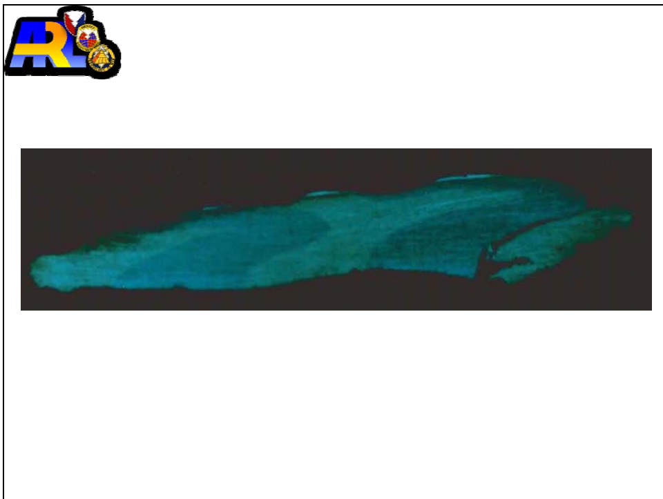
Figure 107. Cross section of a jet particle from alternately layered copper-nickel cone.
