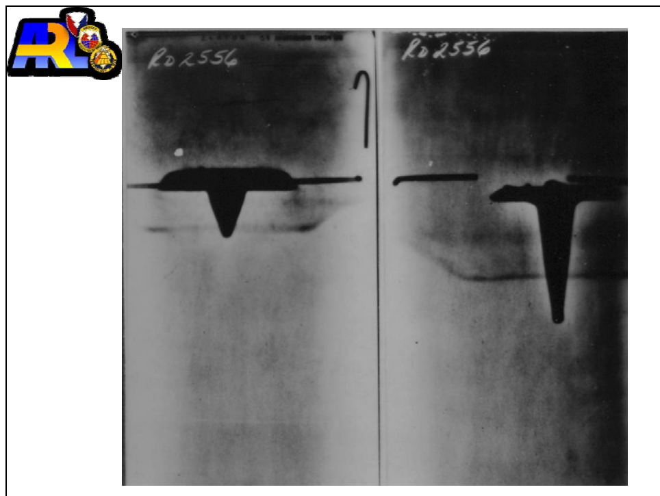
Figure 13. Collapse of a shaped charge with a hemispherical liner (continued).
