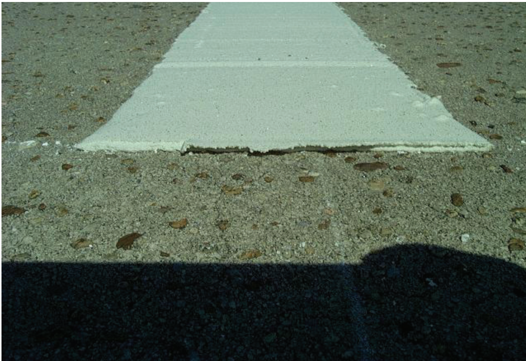
Figure 1. End-on view of PermaStripe™ line from Test 1 at Tyndall AFB showing thickness.
