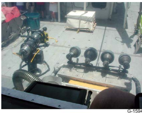
Figure 1. View from inside the Johnson-SeaLink sphere showing the HMI lights mounted far forward on the lid of the work basket. The two inner lights are fitted with filters that transmit blue light, while the outer two are fitted with filters that transmit ultraviolet. The two pairs can be illuminated separately. To the left is the JSL video camera fitted with a yellow filter for imaging blue-light stimulated fluorescence.
