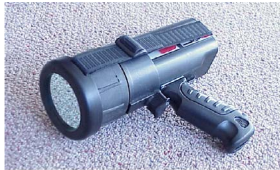
Figure 3. Underwater Kinetics Light Cannon high intensity discharge dive light fitted with a custom interference filter. The light is an effective illumination source for fluorescence exploration and close-range documentation by videotape.
