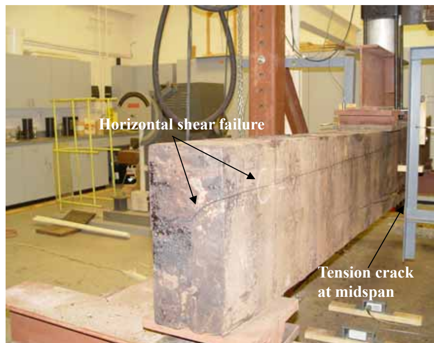
Figure 80. Horizontal shear failure and tension crack on stringer C7.
