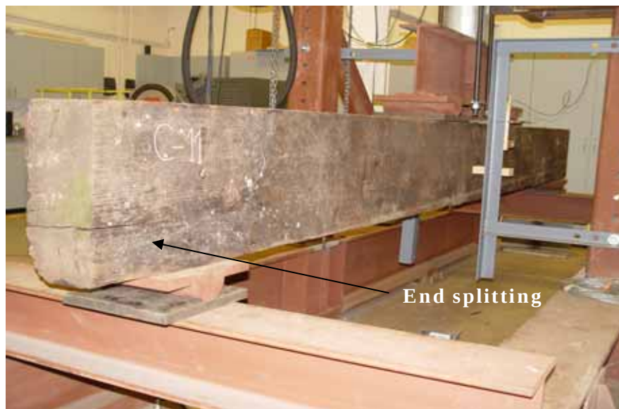
Figure 26. End splitting on specimen C11.
