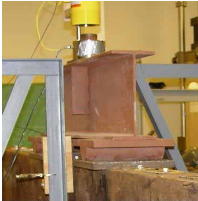
Figure 63. The load cell-hydraulic ram setup with spreader beam.
