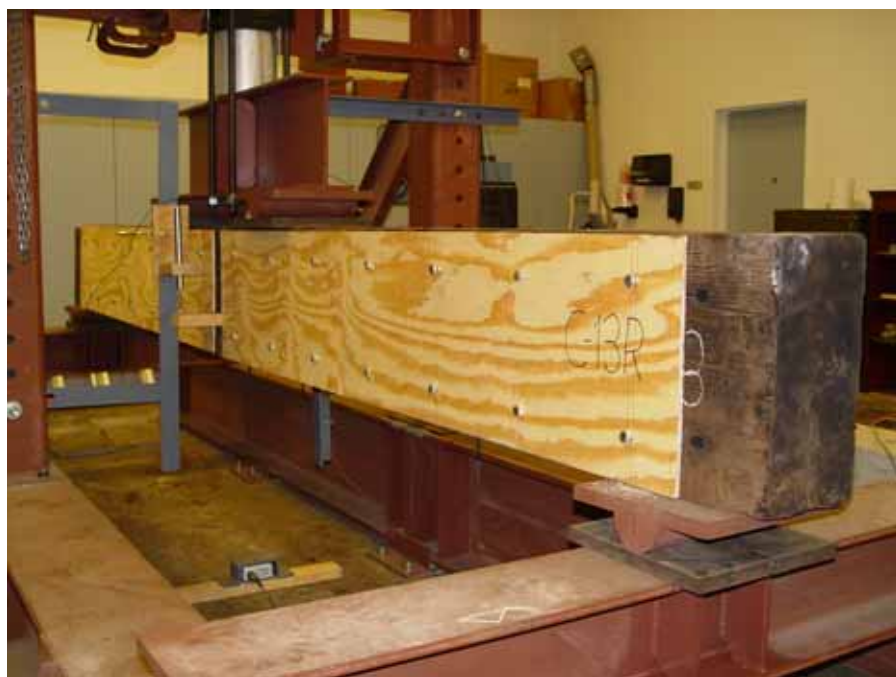
Figure 53. Specimen C13-R repaired with plywood side plates.
