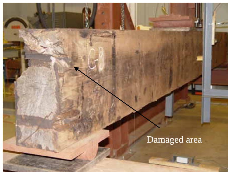
Figure 23. Damaged area at the end of specimen C9.
