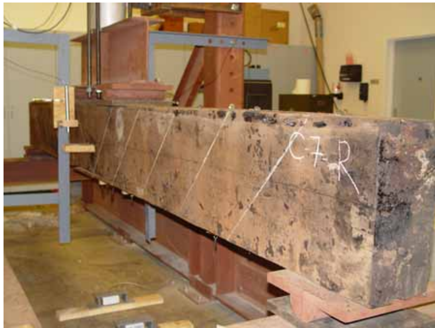
Figure 48. Specimen C7-R repaired with lag screws.
