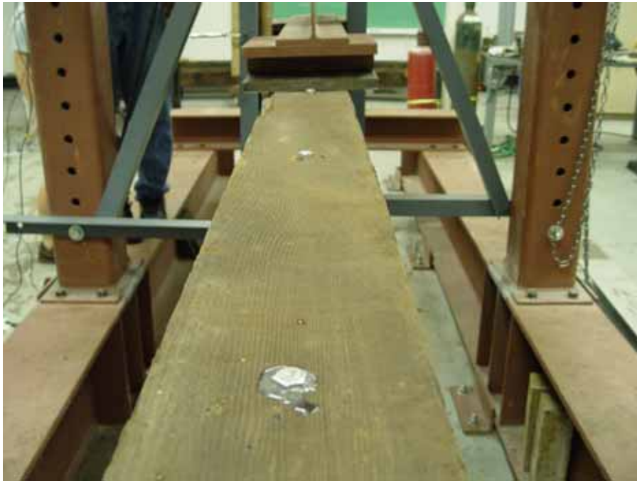
Figure 38. Specimen C3-R repaired using hex bolts and epoxy.
