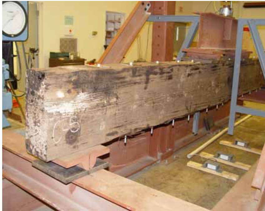
Figure 42. Specimen C5-R repaired with hex bolts and steel plates from top view.
