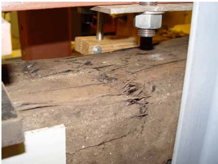
Figure 111. Compression failures due to excessive deformations on stringer C14-R.
