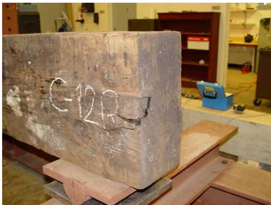
Figure 115. Horizontal shear crack after the failure of stringer C12-R.
