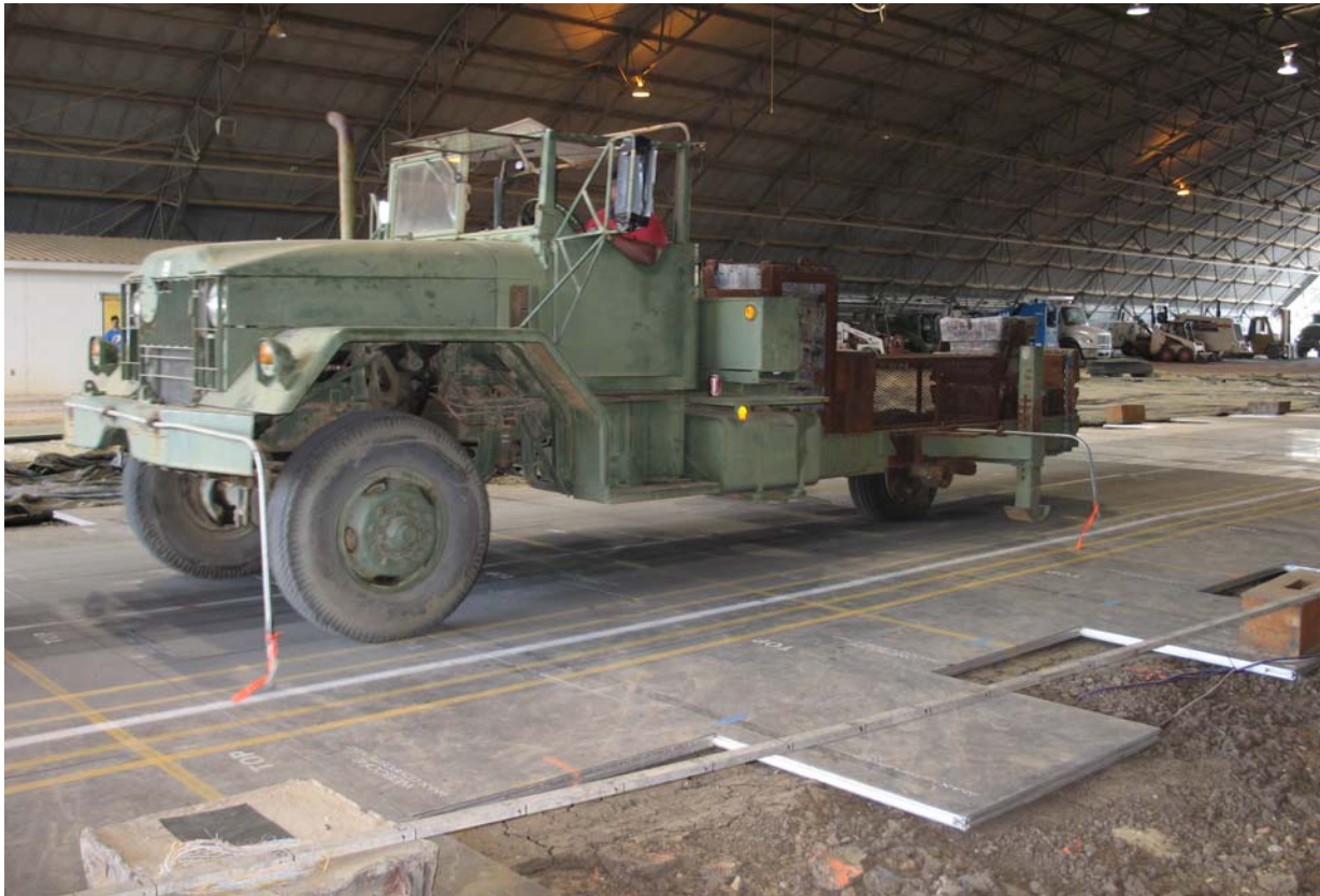
Figure 21: Load cart with full load of 156,725 N (35,235 lbs) trafficking across center of mats
