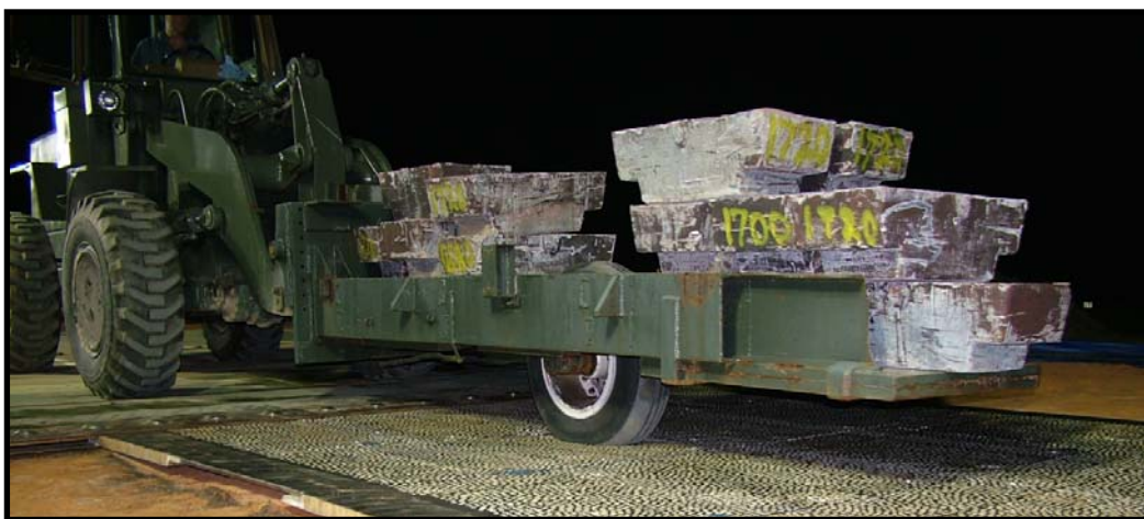
Figure 5: Load cart with F-15E tire and loaded to 133,733N (30,000lb)
