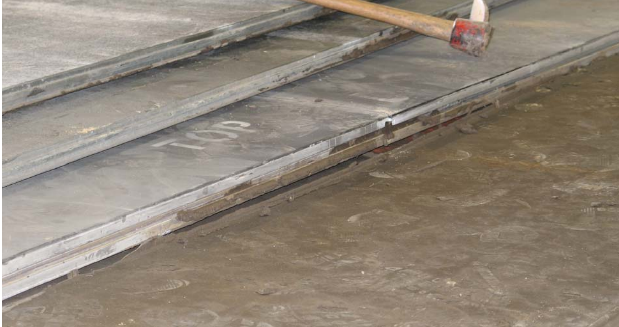
Figure 22: Rutting after pass 384 in test section next to the composite mat test section.
