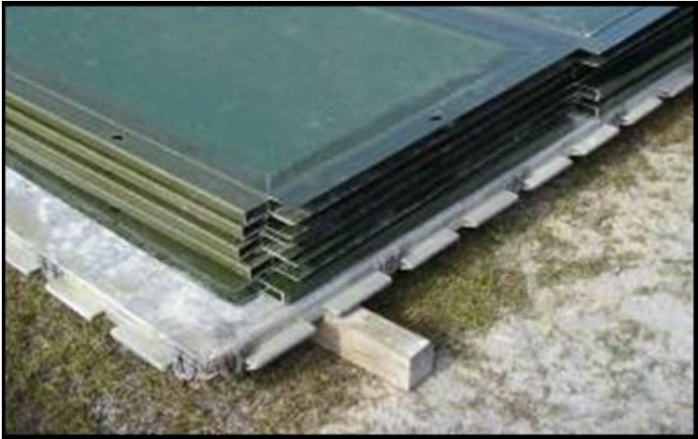
Figure 10: Contractor A panel edge modification from lapped edge to tongue and groove
