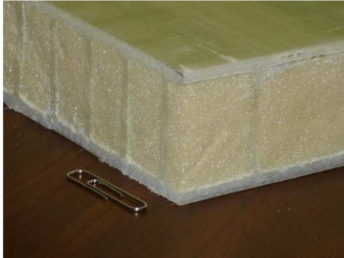
Figure 4: Fiberglass/vinyl-ester face sheets and stitching with foam core
