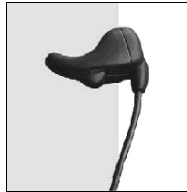
Figure 72. Two hybrid bone conduction communication devices from Savox Communications. (The left panel shows the HS-C and the right panel shows the EC. Both have a bone conduction microphone and an air conduction loudspeaker. The HS-C is designed to be mounted in a helmet and the EC is worn in the ear canal. Downloaded from: http://www.savox.com , October 6, 2006.)
