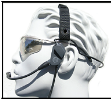
Figure 71. A hybrid bone conduction communication device from Tactical Communication Industries. (The left panel shows the device on a manikin head and the right panel shows the device itself. Downloaded from http://www.tacticalcommand.com , September 20, 2006.)
