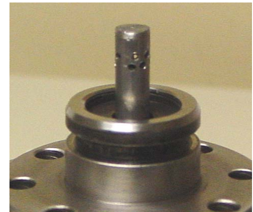
Water Cooled Nozzle with Swirl Coax Element
