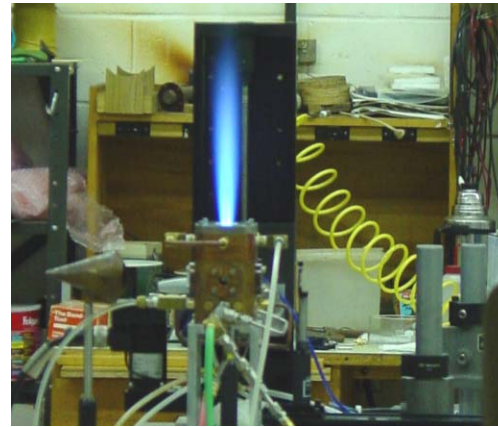
Water Cooled Chamber with Impinging Injector
