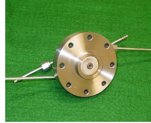
Water Cooled Nozzle with Swirl Coax Element
