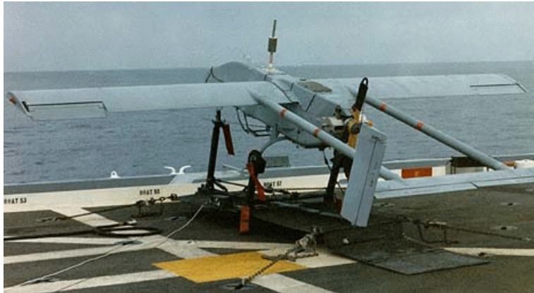
Figure 8. Pioneer Ready To Launch from Ship
