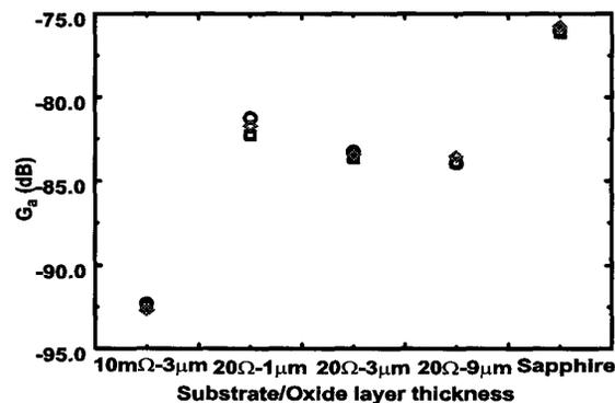
Fig. 10. Antenna gain at 24 GHz vs. substrate resistivity and oxide thickness for 3-mm zigzag antenna pairs. The antenna pair separation is 1 m. It shows three sets of data.
