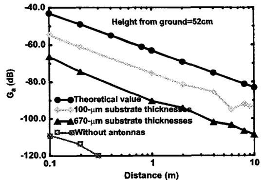
Fig. 6. Antenna gain vs distance in the outdoor dirt environment for 3-mm zigzag antennas on a 20- $\Omega$ -cm substrate with a 3- $\mu$ m oxide layer with 670 and 100- $\mu$ m substrate thickness at 52 cm height. The measurement frequency is 24 GHz.
