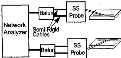
Fig. 4. Antenna measurement setup with a network analyzer.
