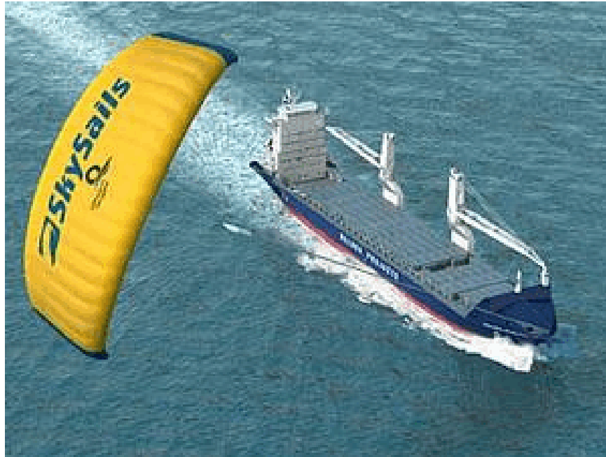
Figure 9. SkySails Concept Applied to Commercial Cargo Ship
