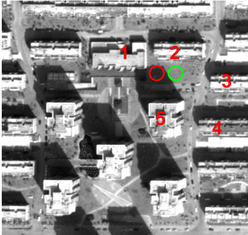
Figure 12. An example of a scene where surrounding buildings can impact the AOD calculations by either reflecting radiance into an ROI or by blocking aerosol scattered radiance into the ROI.
