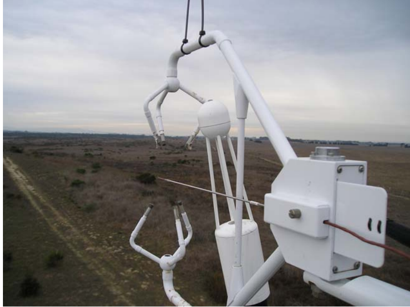
Figure 3. 3-axis sonic anemometer with a fine wire temperature probe extending from the left side of the mount and the open path gas analyzer mounted to the right. (picture by Richard Lind of NPS)
